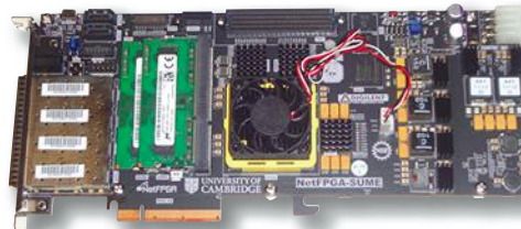
2. Digilent's NetFPGA SUME board connects Xilinx's latest Virtex 7 FPGA to 10 Gbit/s serial connections.
