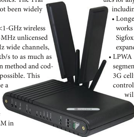
The Systech SL1500 gateway can hold up to five plug-in wireless modules for a mix of Wi-Fi, Bluetooth, ZigBee, Z-Wave, and 3G/4G cellular applications. Ethernet provides the Internet connection.
