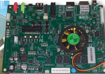
1. The 360-deg. surround view (left) can be experienced using the Renesas R-Car evaluation board (above).
