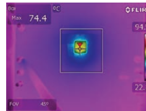
Figure 5. VIN = 5V, VOUT = 3.3V/5A, TA = 25°C Thermals
